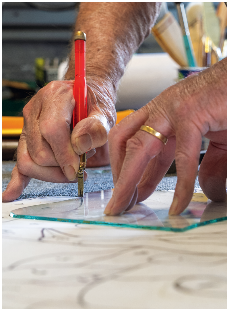
CLOCKWISE FROM TOP: Peter holds up a completed stained glass panel; the broken windows before Peter repaired them in Walcha's St Andrew's Anglican church, featuring some of the earliest stained glass in regional NSW; scoring along a sketched template using a glass cutter.
